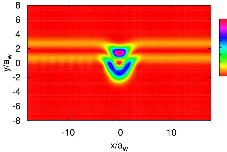
Figure 3; The electron probability density corresponding to the conduction peak in Figure 2.
