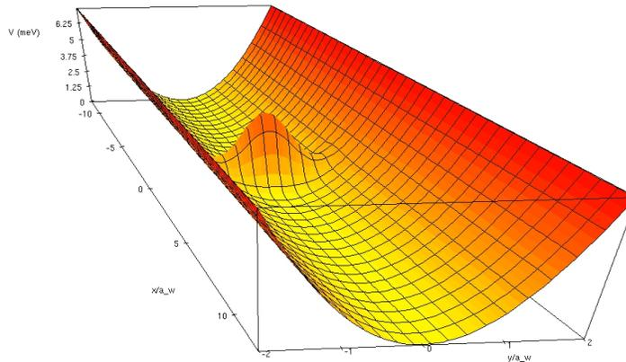
Figure 1, Quantum wire with a repulsive smooth scatterer.
