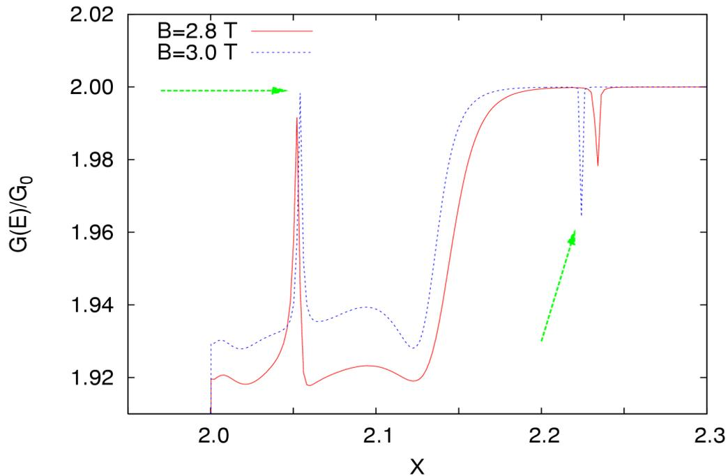
Figure 2; The conductance of the wire with respect to the scaled energy  $X$ , which assumes an integer value each time a new subband opens for transport in the wire.
