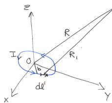
$$\vec{A} = \frac{\mu_0 I}{4\pi} \vec{e}^{-iBR} \left\{ (1 + iBR) \left( \frac{d\vec{l}}{R_i} - iB \int d\vec{l} \right) \right\} = 0$$
