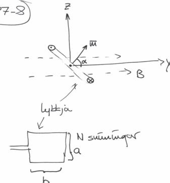
$$\begin{aligned} \text{Vogd á lykju} & \text{er} \\ \bar{T} &= \bar{m} \times \bar{B} \\ &= -\hat{a}_x \text{Nab} I B \sin x \end{aligned}$$
