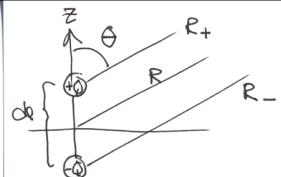
$$\rightarrow V = \frac{Q}{4\pi\epsilon_0} \left\{ \frac{e^{-i\beta R_+}}{R_+} - \frac{e^{-i\beta R_-}}{R_-} \right\}$$
