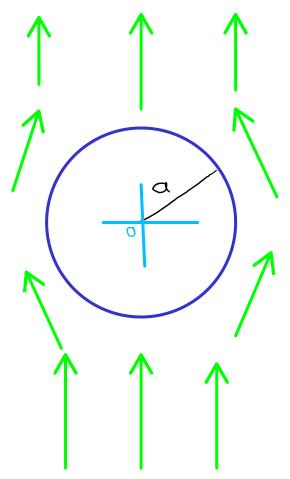
Flow of current around a cylindrical hole drilled into a slab of material. Steady state, so the equation of continuity gives
