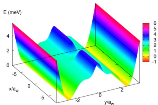
Scattering potential = window between wires
